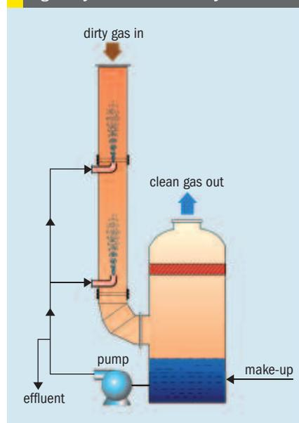
Fig 3: Combined SUPERCLAUS® / DynaWave® process
