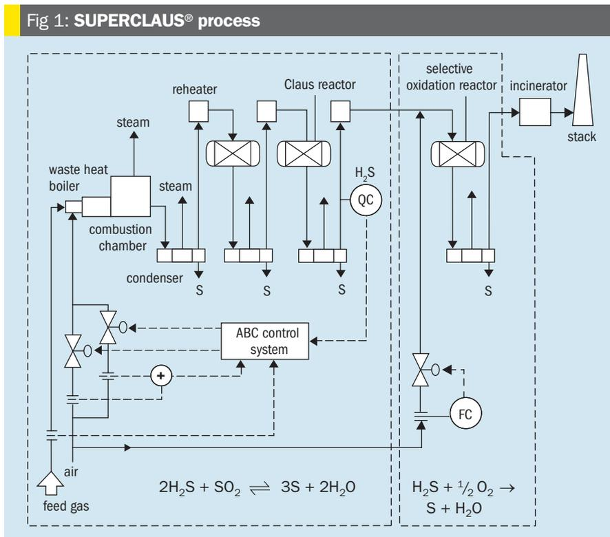
enters the SUPERCLAUS® reactor for selective oxidation of the H<sub>2</sub>S to elemental sulphur. The formed sulphur is then condensed and recovered by the SUPERCLAUS® condenser. Tail gas from the SUPERCLAUS® stage is typically routed to an incinerator for thermal oxidation of the residual sulphur components and venting of the flue gas to atmosphere via the incinerator stack.
