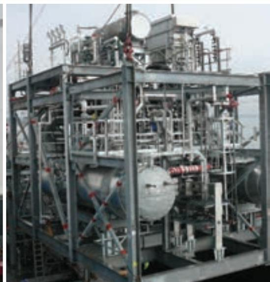
based on Jacobs' Comprimo® proprietary desulphurization technology, SUPERCLAUS®, and delivered by Jacobs. Previously, waste gases from the refining process were burned off in furnaces, releasing sulfur dioxide into the atmosphere. In the new design, WGT compressors divert these gases to the SRU, which removes the sulfur and produces clean flue gas.
